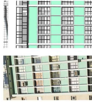
EXISTING A/C WINDOW UNITS WILL BE REMOVED AND NEW COMPATIBLE STEEL WINDOWS TO BE PROVIDED
