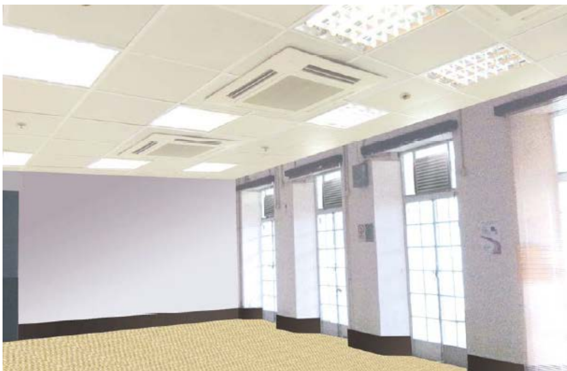
Figure 10 Artist impression of one the training rooms on the G/F with the new false ceiling maintaining at 3.4m from the floor level
