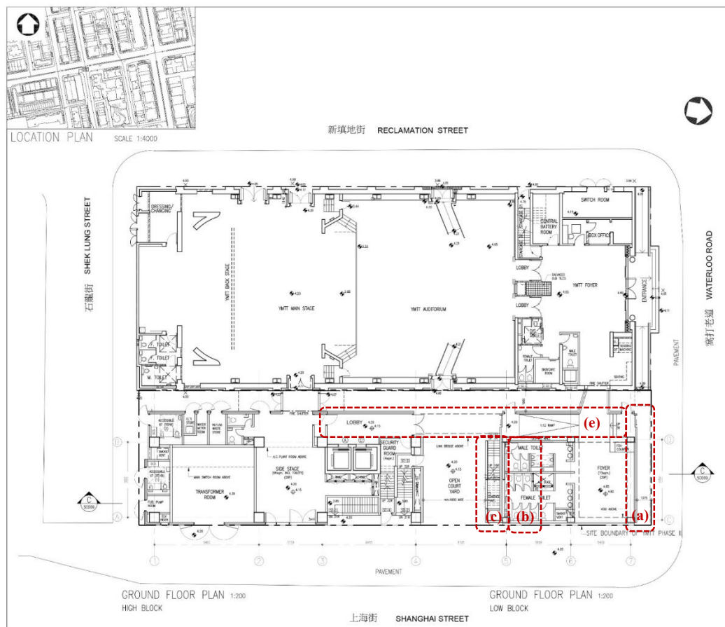
Figure I. Proposed Ground Floor Plan (Low Block) - (a) the frontage of the proposed low block is set back by approximately 1.1m; (b) & (c) the internal staircases and lift core are removed and replaced with an external open staircase leading to landscape roof to provide more space on G/F; (e) the circulation is designed to enhance the appreciation of the east elevation of YMTT.
