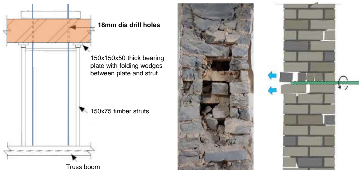
Figure 18 – Slender and cracked brick piers in poor condition remain standing (supported by temporary works), and substantial repairs will be required in recovery work
