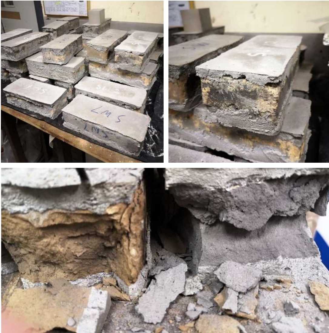
Figure 12 – Forty brick samples were collected for compression tests with results showing that the characteristic compressive strength of the bricks was only 4.32 N/mm 2
