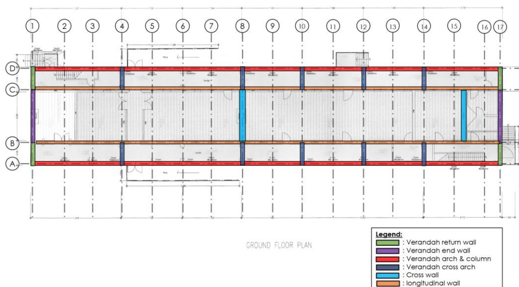
Figure 3-64 2013 G/F record framing plan, with different type of brick walls highlighted in colour dotted lines (Source: Architectural Services Department, Structural Appraisal Report 2013 , with Author's edition)
