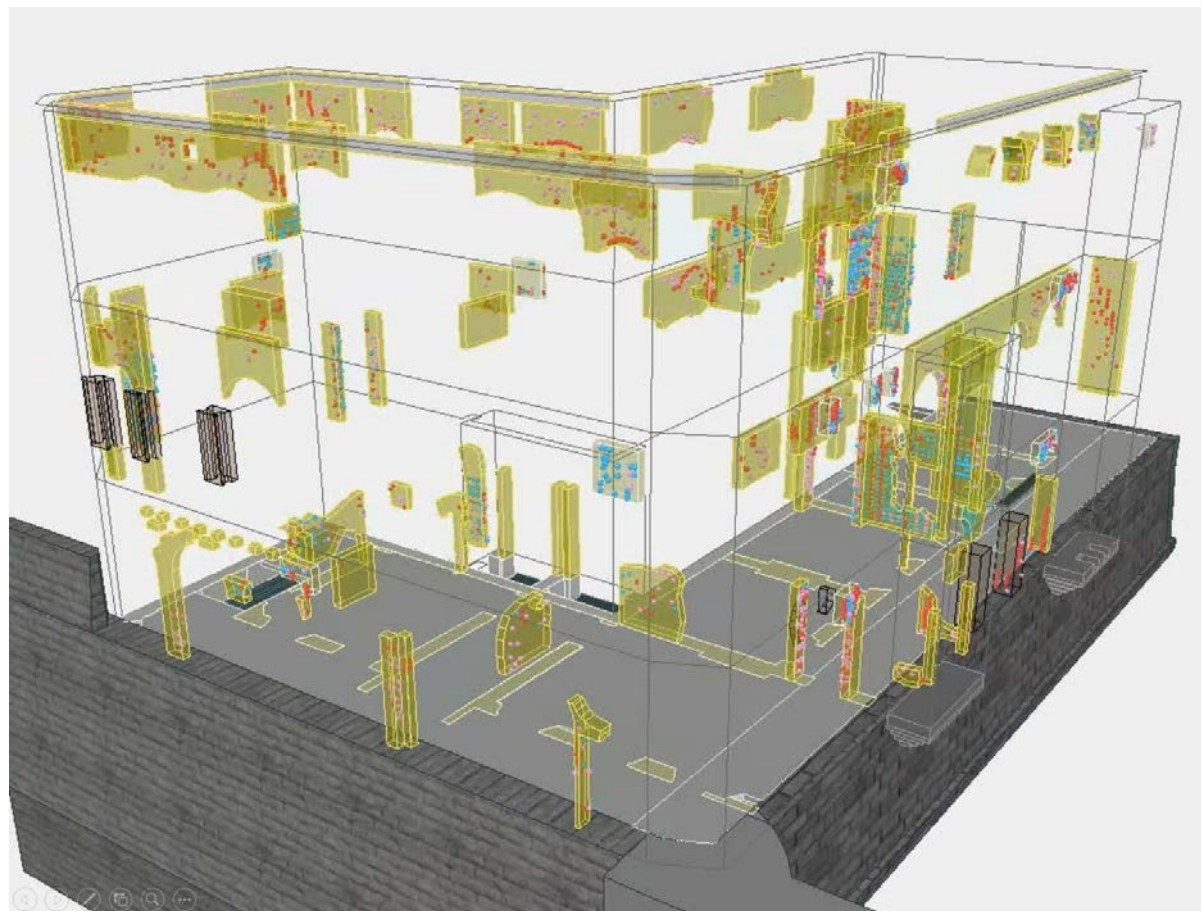
Figure 11 – Consistent types of defects seen in most areas of exposed brickwork
