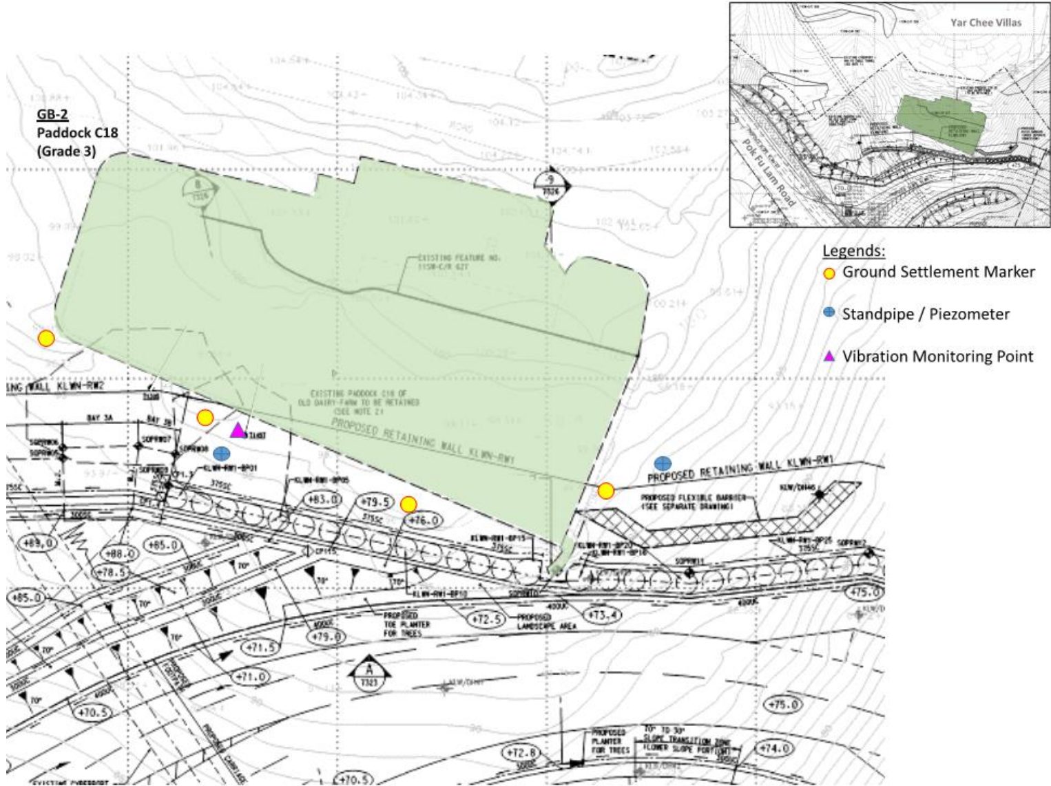
Figure 8 Indicative Locations of Monitoring Instruments (Subject to further detailed geotechnical design)
